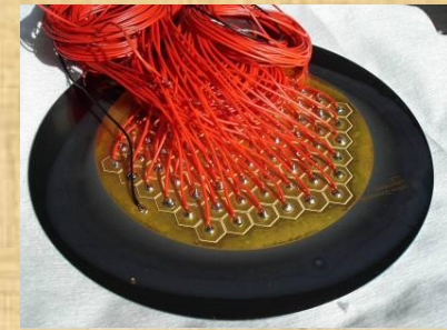
Soldered control and mass wires
